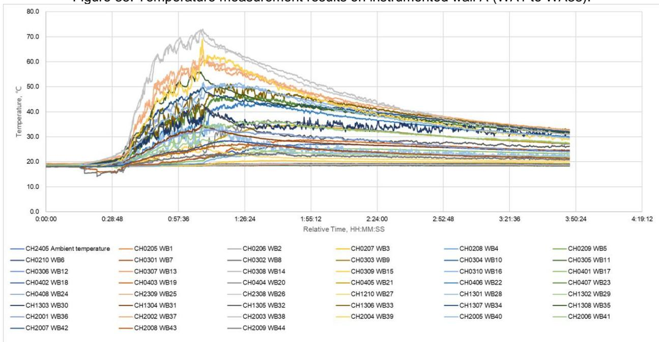
Figure 36. Temperature measurement results on instrumented wall B.
