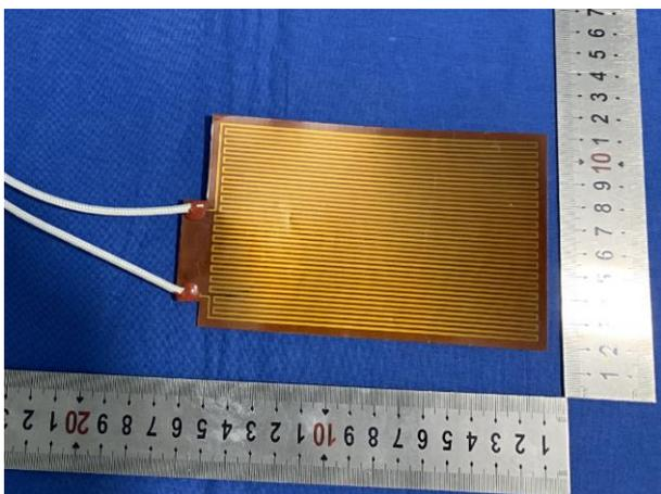
Figure 10c. View of external film heater.
