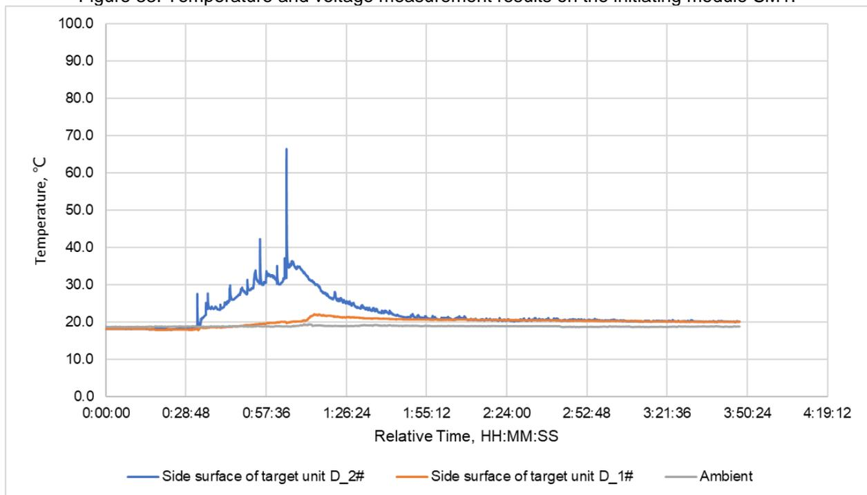
Figure 34. Temperature measurement results on target unit.
