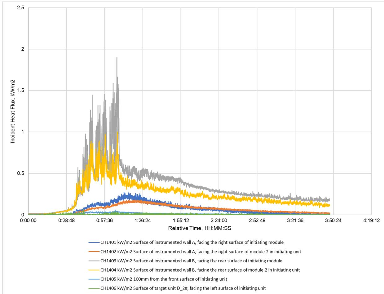
Figure 14. Incident heat flux on instrumented wall surfaces, target unit and front of initiating unit.
