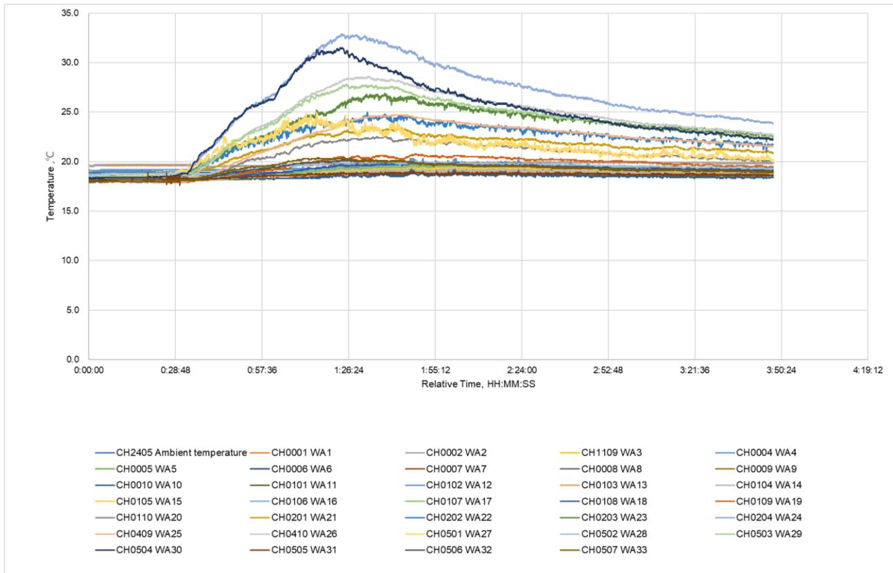
Figure 35. Temperature measurement results on instrumented wall A (WA1 to WA33).
