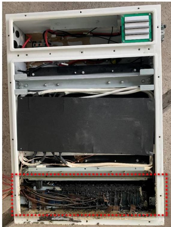
Figure 32b. Photo 01 of thermal runaway location.
