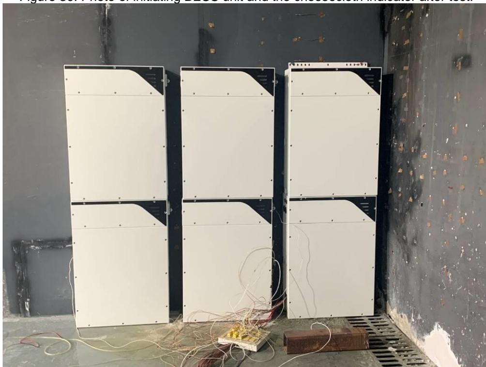
Figure 31. Photo of initiating and target BESS units after test.
