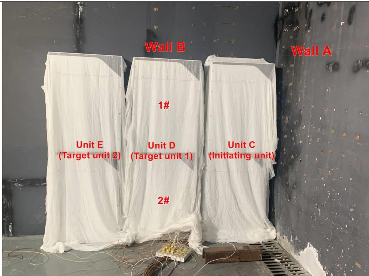
Figure 12. View of BESS units within test room.
