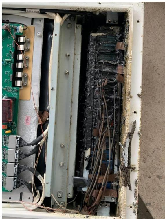
Figure 32d. Photo 03 of thermal runaway location.
