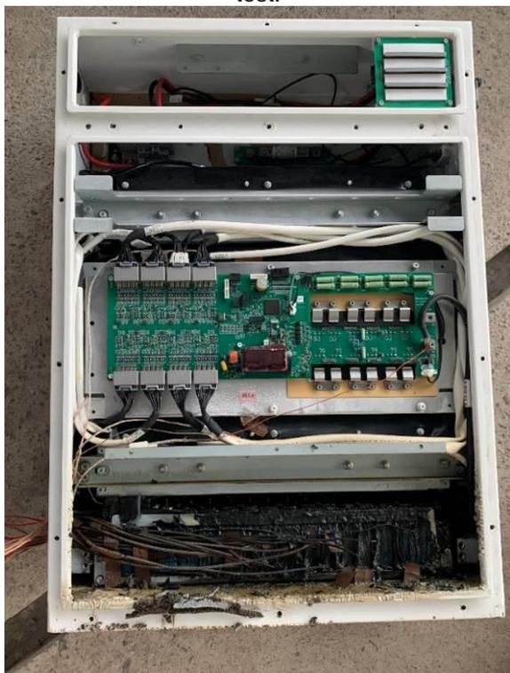
Figure 32c. Photo 02 of thermal runaway location.
