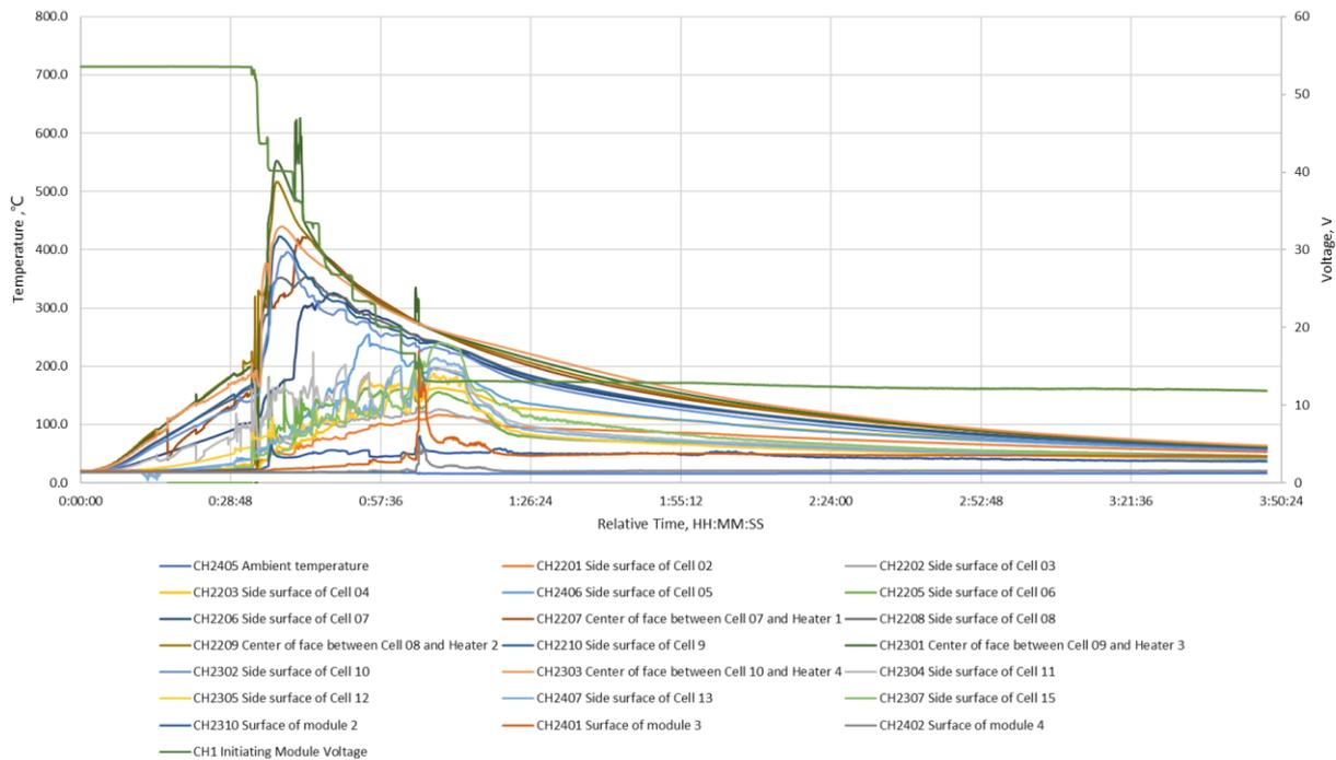
Figure 33. Temperature and voltage measurement results on the initiating module SM1.
