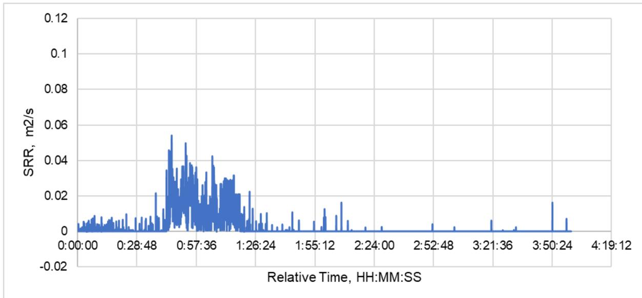
Figure 15. Smoke release rate versus time
