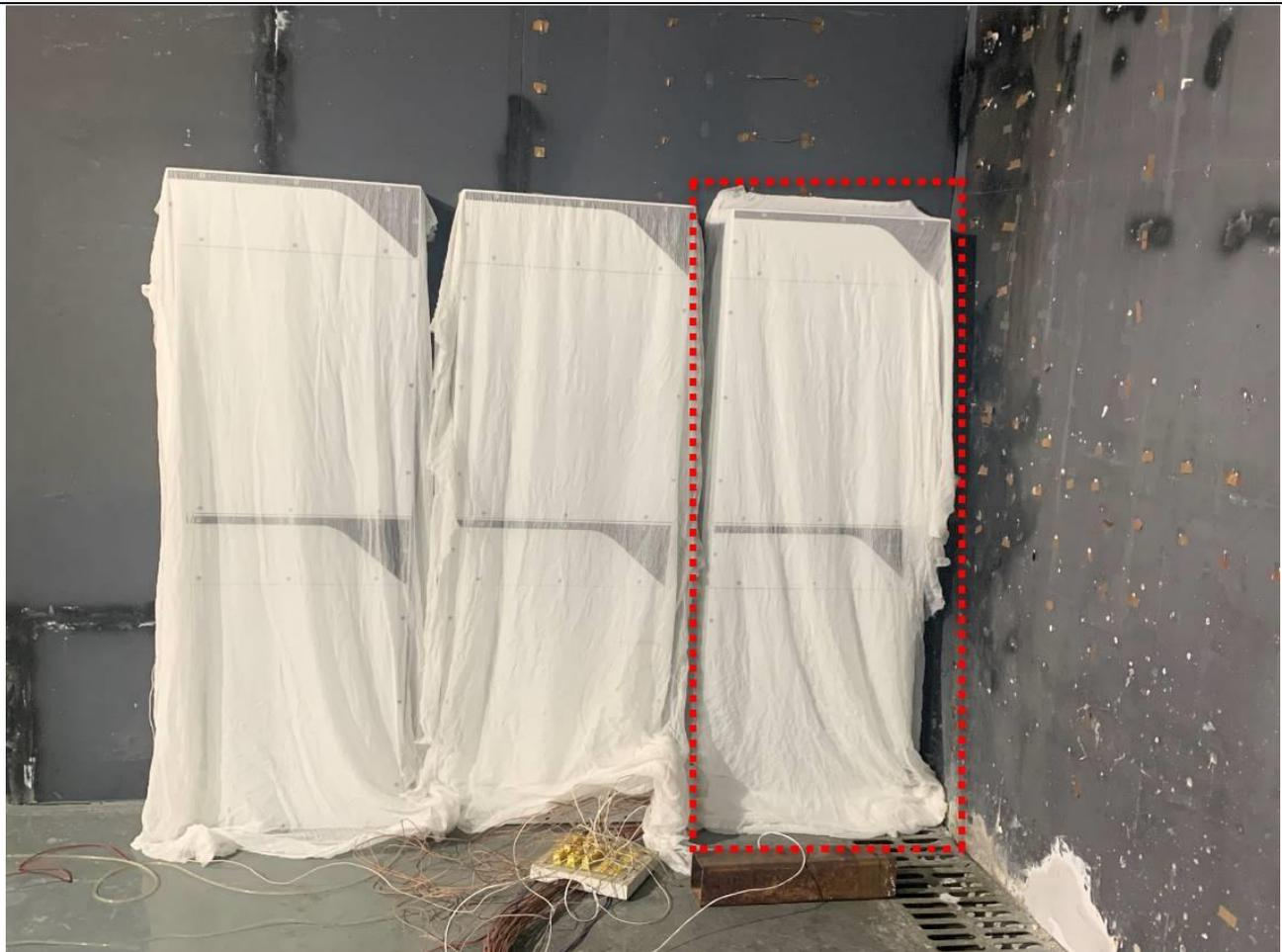
Figure 8. View of the initiating BESS unit before test
