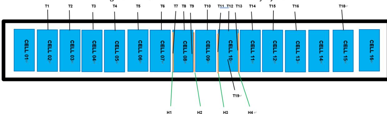
Figure 11b. Schematic illustration of film heaters and thermocouple locations in the initiating module SM1(T1 to T16, T18 means thermocouples T1 to T16, T18. H1 to H4 means Film heater 1 to Film heater 4. View from top.)
