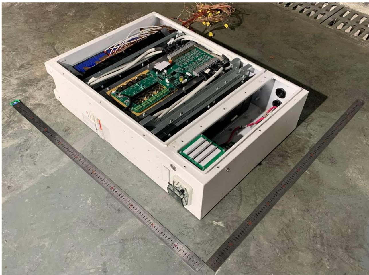
Figure 9. Internal view of the initiating BESS unit before test
