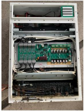
Figure 32c. Photo 02 of thermal runaway location.
