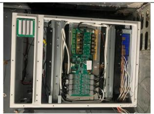
Figure 10a. Internal view of initiating battery system.
