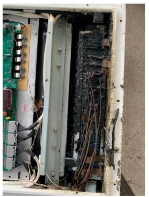
Figure 32d. Photo 03 of thermal runaway location.
