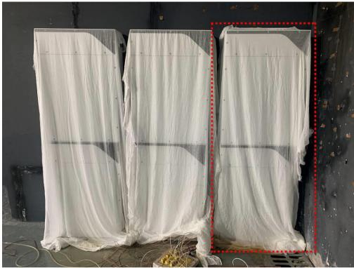
Figure 30: Photo of initiating BESS unit and the cheesecloth indicator after test.
